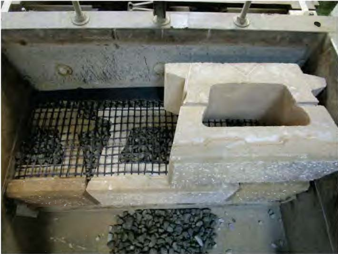
Figure A-2. SF20 geogrid / ShoreLoc block connection test setup.
