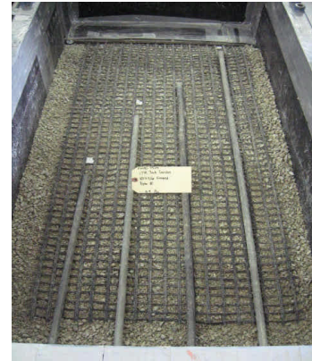
80 kN/m Geogrid @ 20 kPa Post-test
