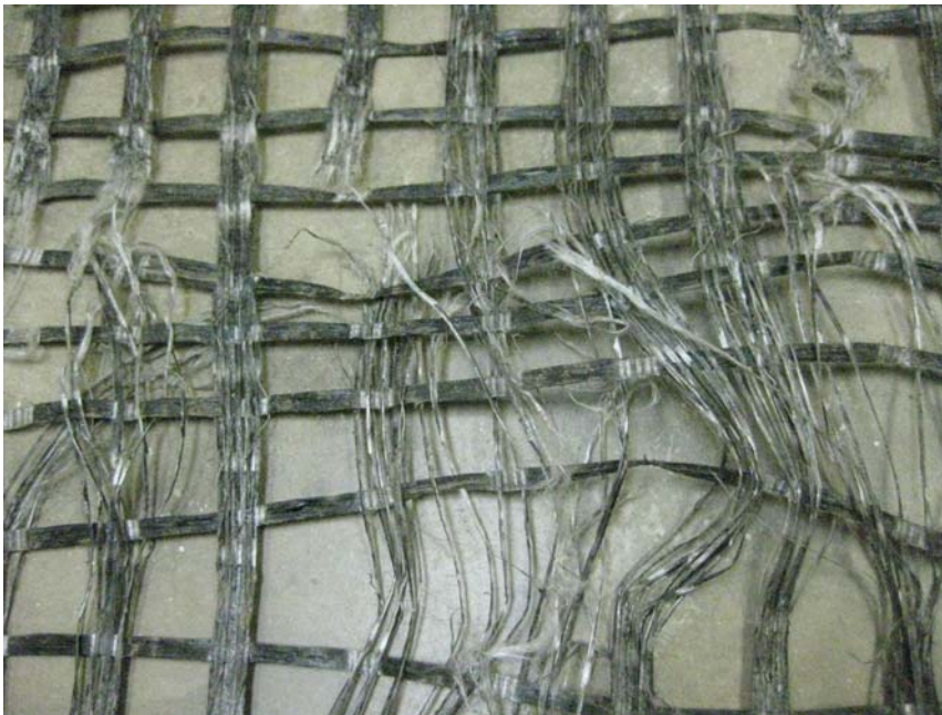
Figure A-4. Junction failure (sliding of a XD rib along MD ribs) and rib rupture of CTMGGU 80 geogrid at the completion of test #3G at 4800 lbs/ft normal load.
