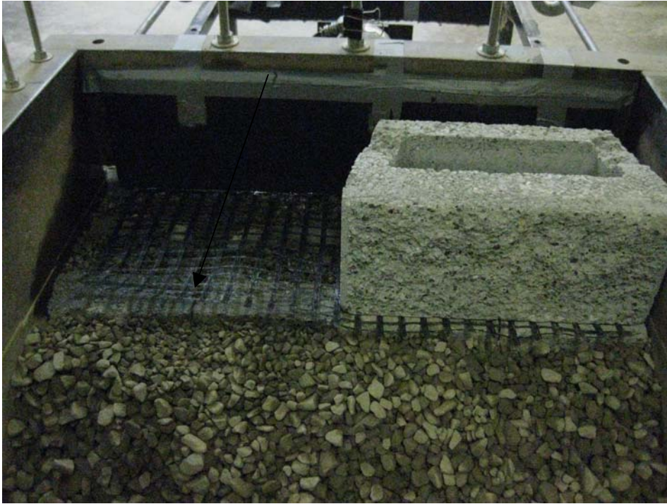
Figure A-2. Connection test setup.
