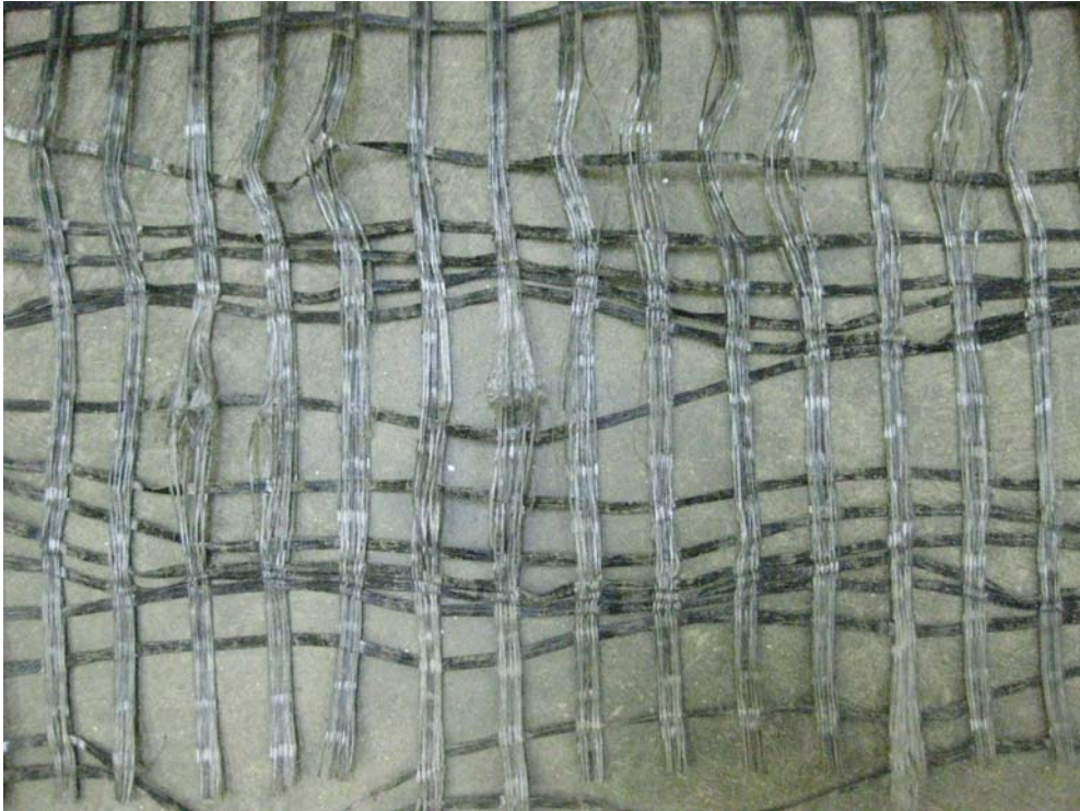
Figure A-4. Junction failure (sliding of a XD rib along MD ribs) of CTMGGU 60 geogrid at the completion of test #2C at 1125 lbs/ft normal load.
