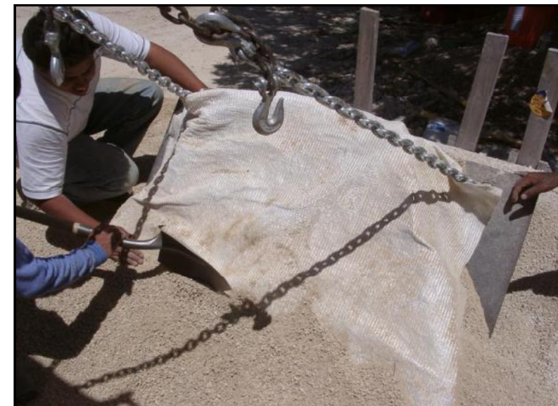
THE STEEL PLATES ARE TILTED TO FACILITATE EXHUMATION
