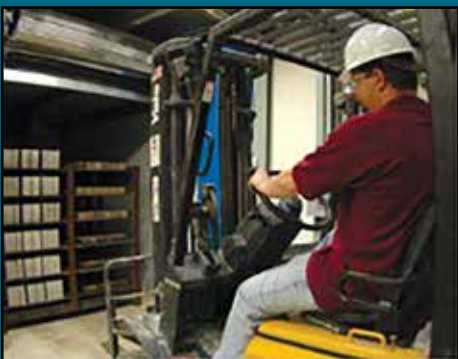
Figure 7. Product Placed in Kilns for Curing
