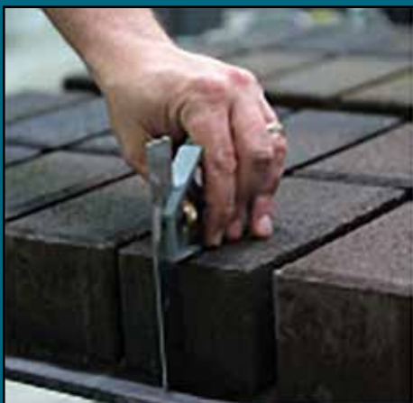
Figure 6. Manual Height Consistency Check During Production
