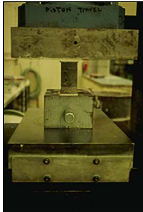
Figure 8. SRW Coupon Capped for Compressive Strength Testing
