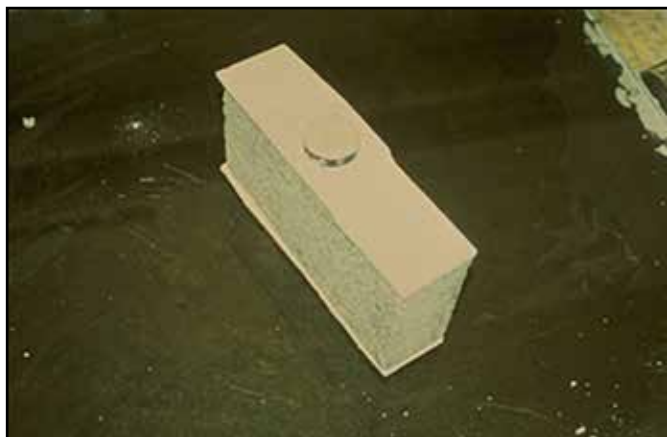
Figure 8. SRW Coupon Capped for Compressive Strength Testing
