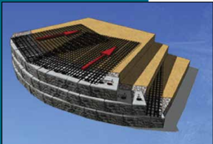
Figure 5. Example of Manufacturer Recommendations for Curves
