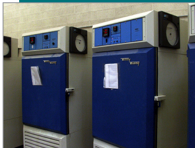
FIGURE 9 FREEZE THAW TESTING CHAMBER (NCMA PHOTO)
